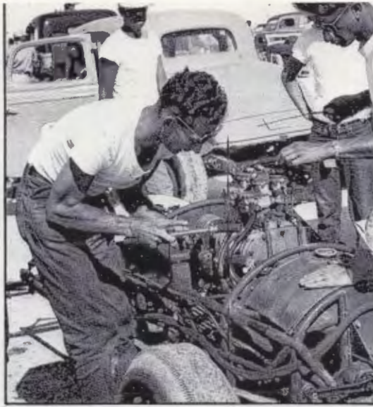
For many years the most powerful flathead by far was Tom Beatty's GMC-blown tube-frame belly tank, which turned 199 at El Mirage, 212 at Bonneville. Here Tom checks the plugs of an early version, while engineer Barney Navarro checks the oil for telltale signs of bearing dust. Tom blew up a lot of engines trying to improve on these speeds; used to bring his boring bar, extra blocks, and boxes of parts to Bonneville and build complete engines on the steps of the Western Motel. Peterson
