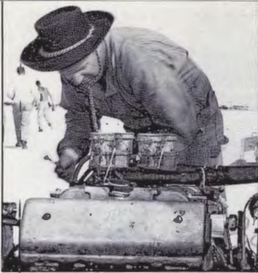
Arnold Birner tunes the converted Mercury using his heads in a belly tank which reached over 140 mph at Bonneville.
