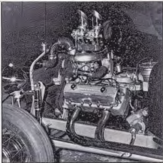
A very wild street engine using Alexander heads and a modified Schwitzer-Cummins centrifugal blower. Alexander heads had poor porting, gave cooler running than a standard flathead but not much more power. Peterson
