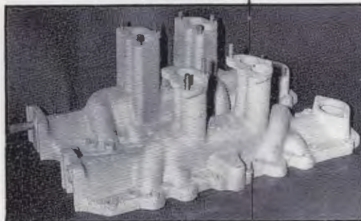
Edelbrock "Regular manifold replaced the pre-war "Sling-shot" design about late 1946, was in turn replaced by another model (in rear) about 1949. All three were among the best dual manifolds for street use. Dees
