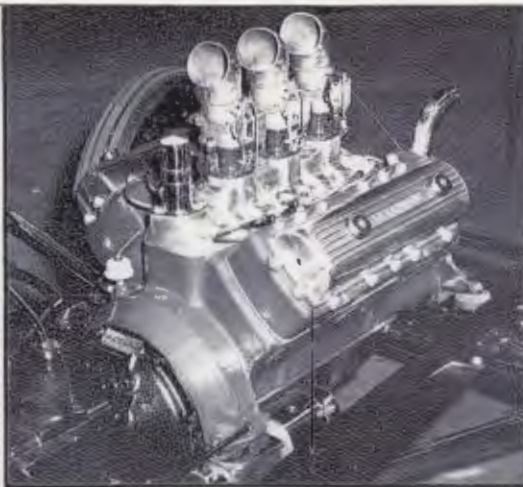
Another shot of an Alexander conversion makes it clear that the intake system remained standard—in the block—while only the exhaust came through the head. This "F" head arrangement is the reverse of all others, such as Rolls-Royce, Willys, and Riley fours, in which the intake was routed through the head. Peterson
