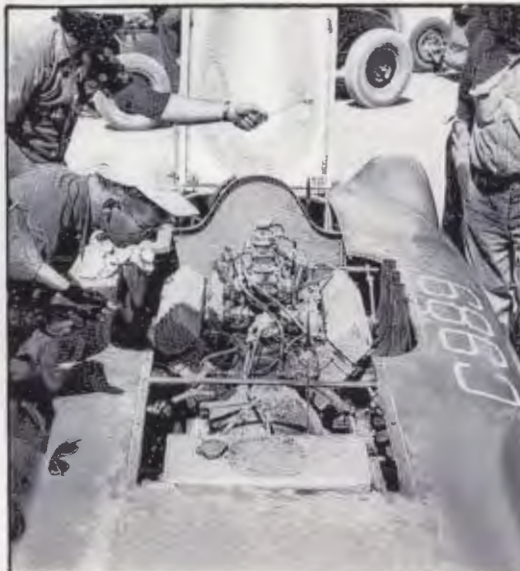
Al Barnes used a set of the rare Cummings overheads on a 21-stud block in his beautiful street roadster, and there are another set or two in use. Al built a fuel injection system for this car also. Peterson
