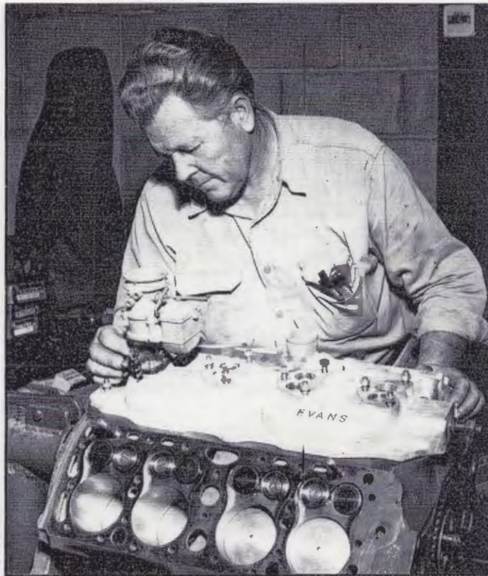
Closeup of a racing head shows machine work for low-dome pistons and pockets for the valves. Ideally the flycuts should be at exactly the same angle as the valve heads, so that clearance can be reduced to the absolute minimum. The valve heads may then hit the combustion chamber roof with no damage in extreme RPM situations.
