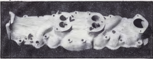
Dave Burns produced this low-riser manifold in 1941 and also supplied risers which could be bolted on to provide generator clearance. This excellent design was made after the war with a different style of lettering in place of the raised block type shown here.
