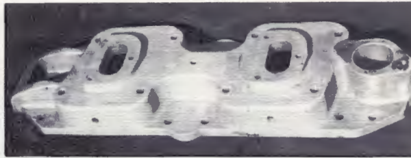
One of the earliest cast aluminum dual manifolds for the flat-head was made by Robert M. Roof, of Anderson, Indiana, who eventually made a full line of V-8 engine and chassis equipment. This particular manifold design is very poor, but was produced until the late Forties.
